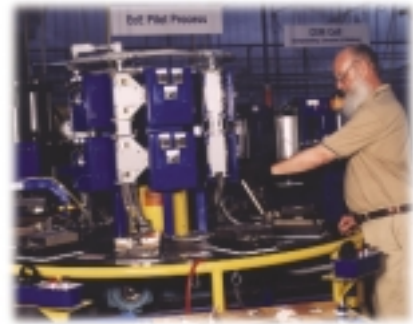
Molds filled with EcE compound are loaded and unloaded during the curing cycle by a ten-station rotary press custom designed for a more flexible and cost-effective process.
