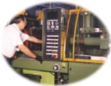
High-volume production processes use a 60-ton injection molding press with a cold runner system for multi-cavity molds to reduce cycle times and material loss.
