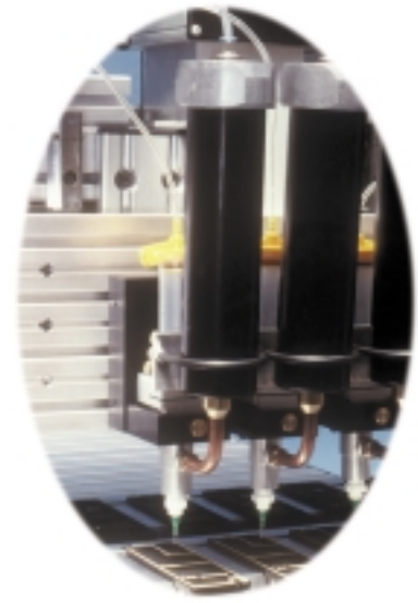
Computerized XYZ form-in-place dispensing machines deposit conductive elastomer compounds onto miniaturized thin wall multicompartment housing covers.
