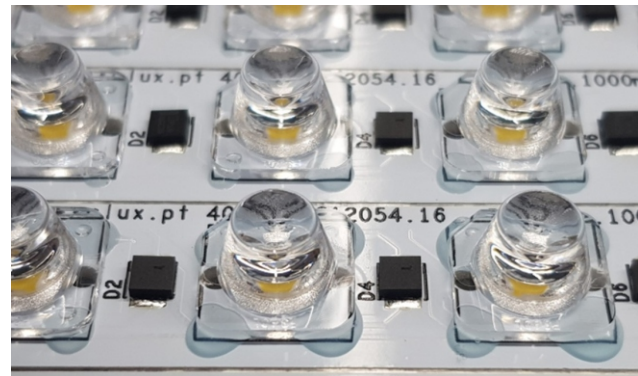
Abchimie 9030 UV UV Glue used for a customer working in lighting to glue lenses on LEDs
