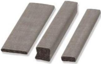
Laird's Fabric-over-Foam 779 EMI gaskets provide wide compression ranges, and excellent EMI shielding performance for customers where EMI issues occur. The 779 EMI gaskets are composed of electrically conductive fabric wrapped around a foam core. They are supplied with a conductive pressure sensitive adhesive (PSA). The Fabric-over-Foam 779 EMI gaskets series is a halogen-free product with cross-section profiles of rectangle.
