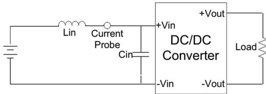
**Output Ripple & Noise Measurement Test**
