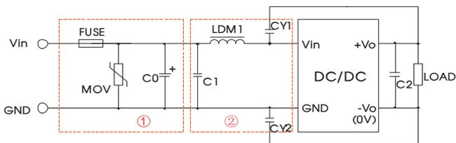
Notes: Part ① in the Fig. 3 is used for EMS test and part ② for EMI filtering; selected based on needs.
