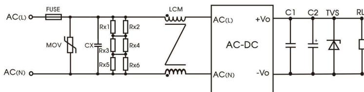
Fig. 2: EMC application circuit with higher requirements
